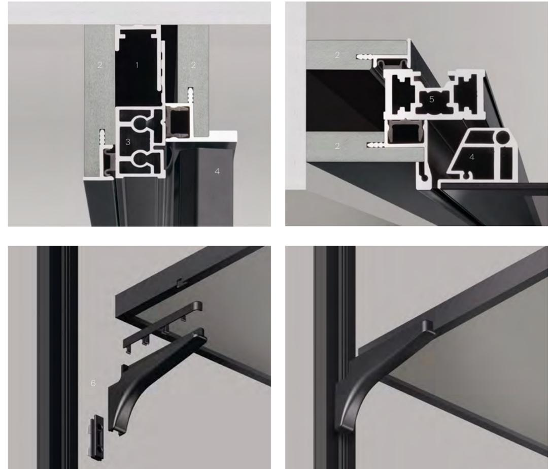
1. Ceiling adjusting profile in extruded aluminium. It allows a perfect leveling of the upright and to compensate any possible unevenness of the ceiling.
